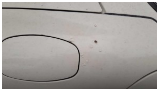
Corrosion aile AVG
